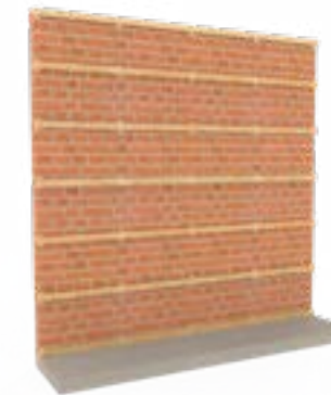
Timber battens straight onto wall
