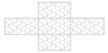
A-B Repeat Type - This type of pattern repeats every other panel. Because of this an "A" and a "B" version of the pattern is manufactured and labeled accordingly. The two versions of the panel are then alternated in the final installation in order to achieve a monolithic appearance.
